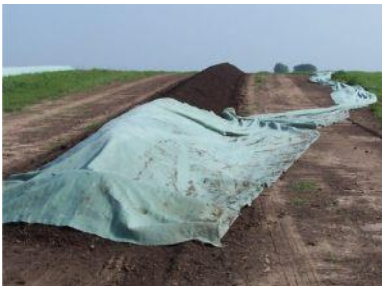
Figure 24: Windrow cover being utilised in an open composting system (source: Midwestbiosystems.com)
