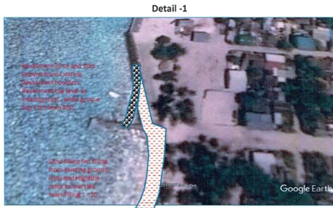
Figure 3: Geo-bag revetment and sand filling area
