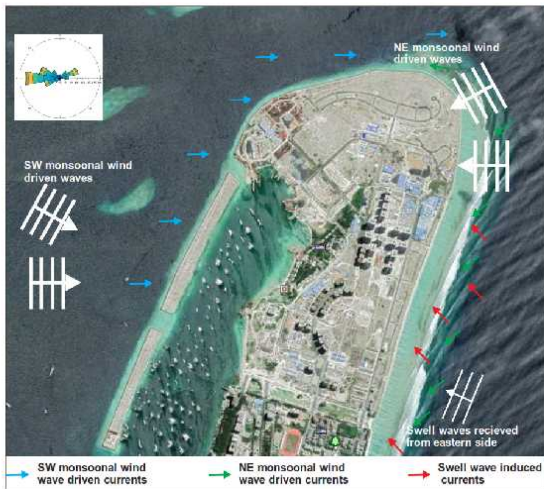
Figure 17: Schematic showing assumed windwave induced currents at the reef system (LaMer, 2020)
