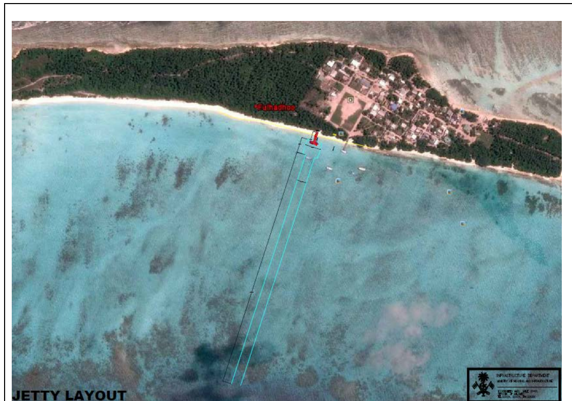
Figure 9: Conceptual drawing and location of the proposed access channel and jetty
