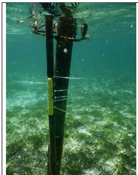
Figure 16: RBR Solo wave measurement device (Wave Gauge) deployed in shallow water
