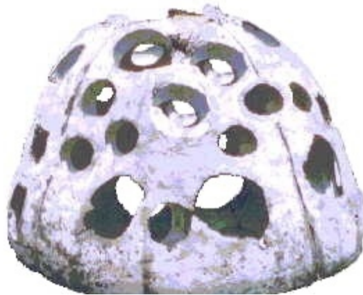
Figure 7: Mould of a reef ball structure - a habitable environment for marine organisms
