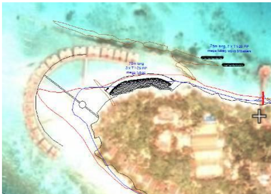
Figure 11: Design of the geo-tube arrangement in the northerneastern part of Fonimagoodhoo.
