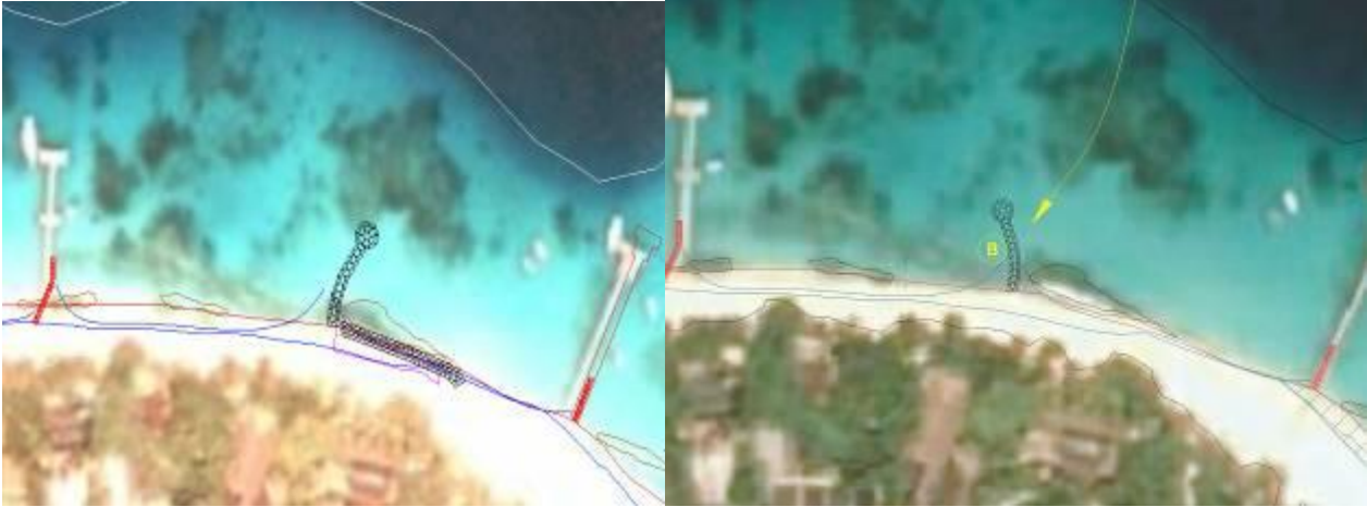
Figure 12: The picture on the left is the new proposed groyne design, and the picture on the right is the old design.
