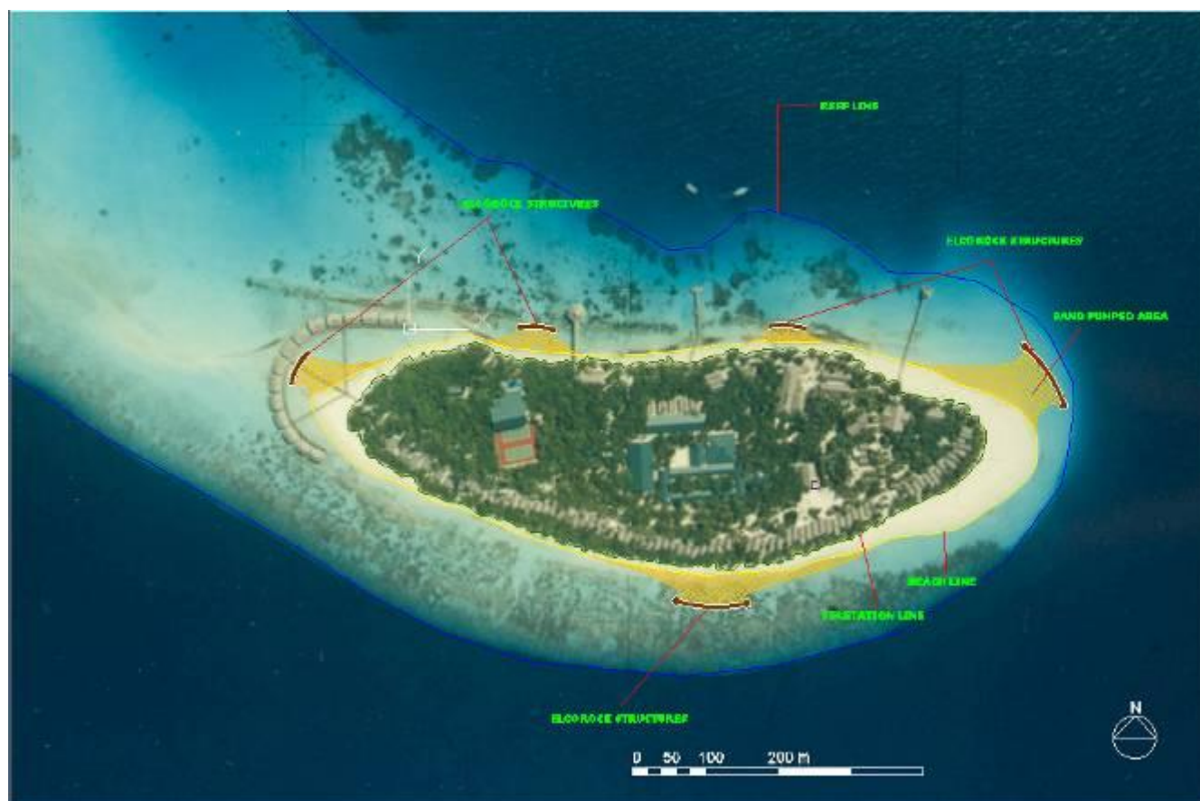
Figure 37: Preliminary design of revetment implementation around Fonimagoodhoo.
