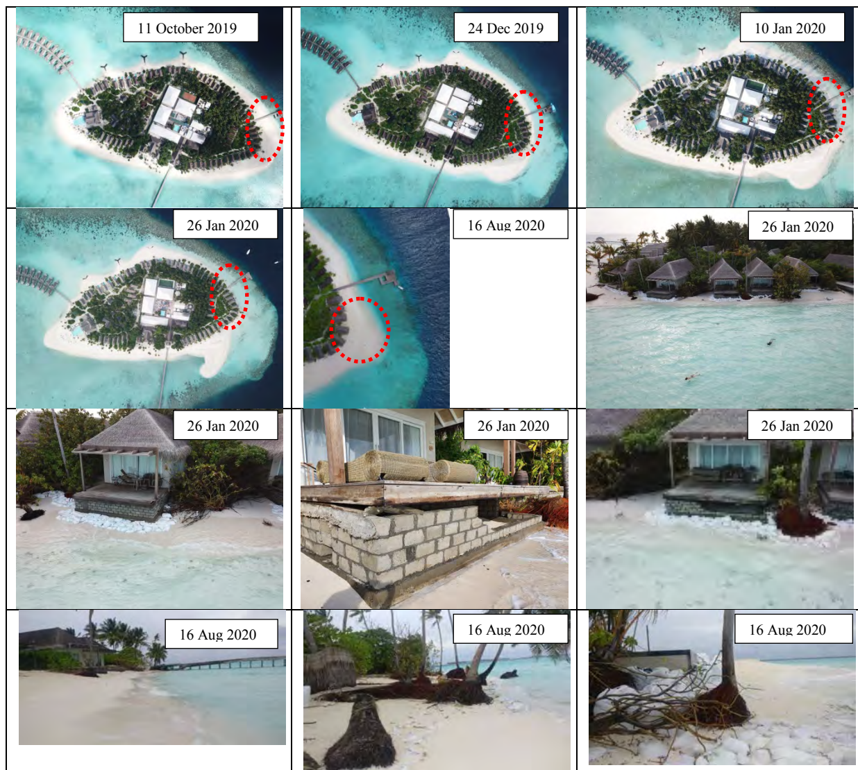
Figure 6. Most recent erosion Magau: time laps photos showing the eastern end beach sand movement and the structural damages near the service jetty area
