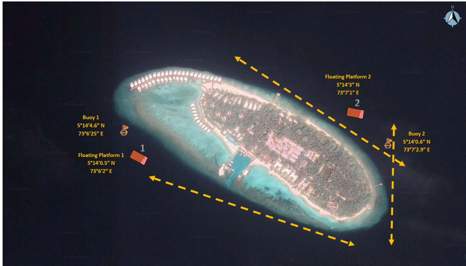
Figure 3.1 Site plan of the proposed platforms (platform 1: location for NE monsoon, Platform 2: location for SW monsoon)
