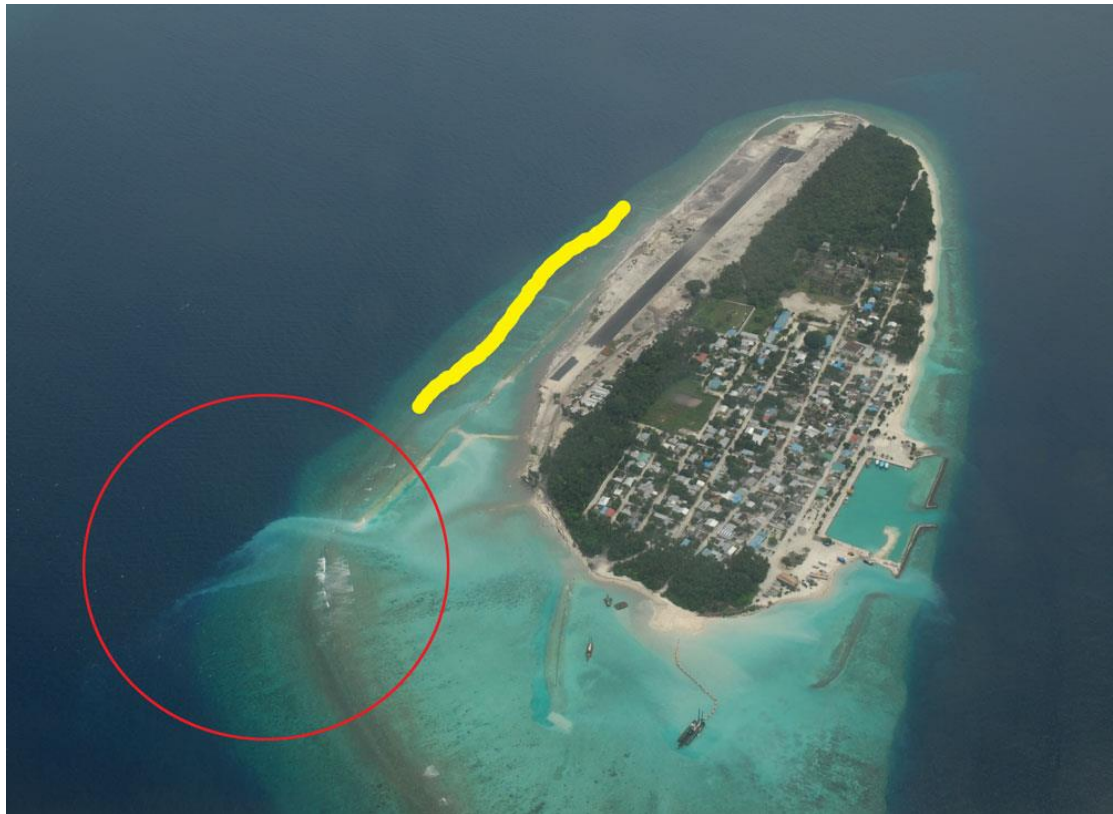
Figure 4: Illustration of how sand bund walls can control sedimentation (Photo: Water Solutions Pvt.Ltd)
