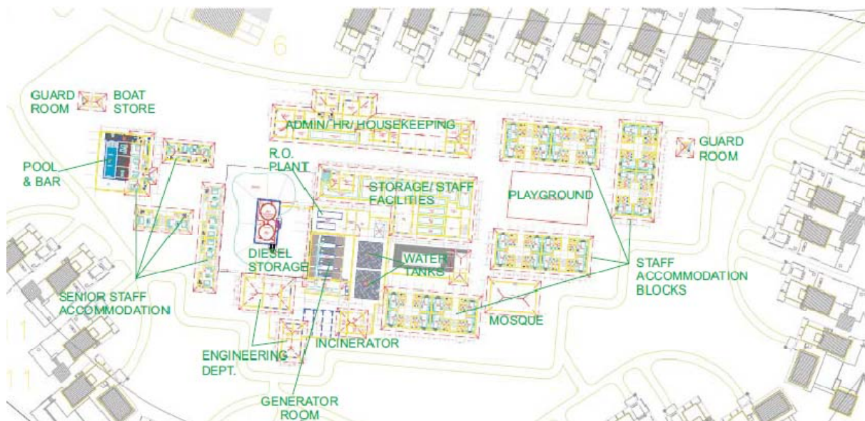
Figure 2.1: Site Layout of the Back-of-the-House Area
